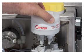
Industry leading Total Cost of Ownership with make up consumption as low as 2ml/hour & service interval up to 18 months/8,000 hours.\*
